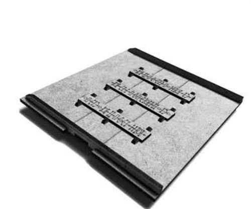
Glue the hook rails into the slots near the edges as shown
