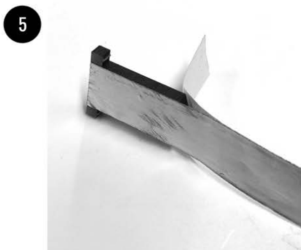
5 Peel backer and stick to the back of each of these three parts. Trim away extra with a razor so that it doesn't overhang.
