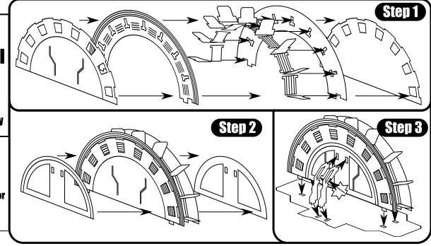
1. Insert striped sheets and tabs into T-shaped slots in the ceter plate on one side and then place the other plate on the other side.
